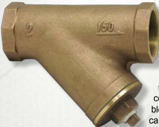
Sure Flow threaded strainers in Cast Bronze feature a machined, tapered seat which ensures a perfect fit for the removable, stainless steel screen. All sizes come complete with NPT blow-off with plug, which can be replaced with a ball valve for on-line blow-down of particulate.
