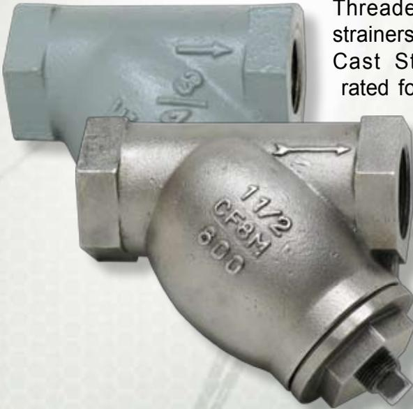
Threaded or Socket Weld strainers in Cast Steel and Cast Stainless Steel are rated for up to 1480 psi for Water, Oil or Gas. A machined, tapered seat ensures a perfect fit for the removable, stainless steel screen. All sizes come complete
