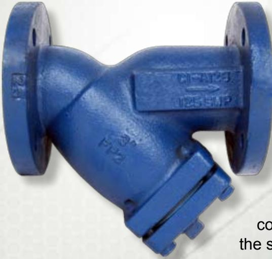
Sure Flow Cast Iron Flanged Strainers feature a machined seat which ensures a perfect fit for the removable, stainless steel screen. All sizes come complete with flanged blow-off cover, gasket & plug. May be installed in vertical or horizontal pipelines with blow-off connection at the lower end of the screen.
