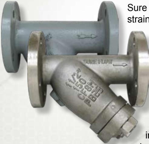
Sure Flow Class 150 ASME Flanged strainers are available in Carbon Steel and Stainless Steel. A machined, tapered seat ensures a perfect fit for the removable, stainless steel screen. Size 2" and larger come complete with flanged blow-off cover, gasket & plug. 1 1/2" and smaller come complete with solid threaded cover and gasket. May be installed in vertical or horizontal pipelines with blow-off connection at the lower end of the screen.
