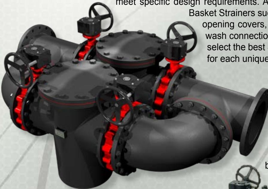
Sure Flow Model BDB Dual Basket Strainers are a bolted design. The standard version comes in Cast Iron material with Class 125 flanged connections and is available in sizes 2" through 18". Baskets can be supplied with bolted or quick release clamp covers.
