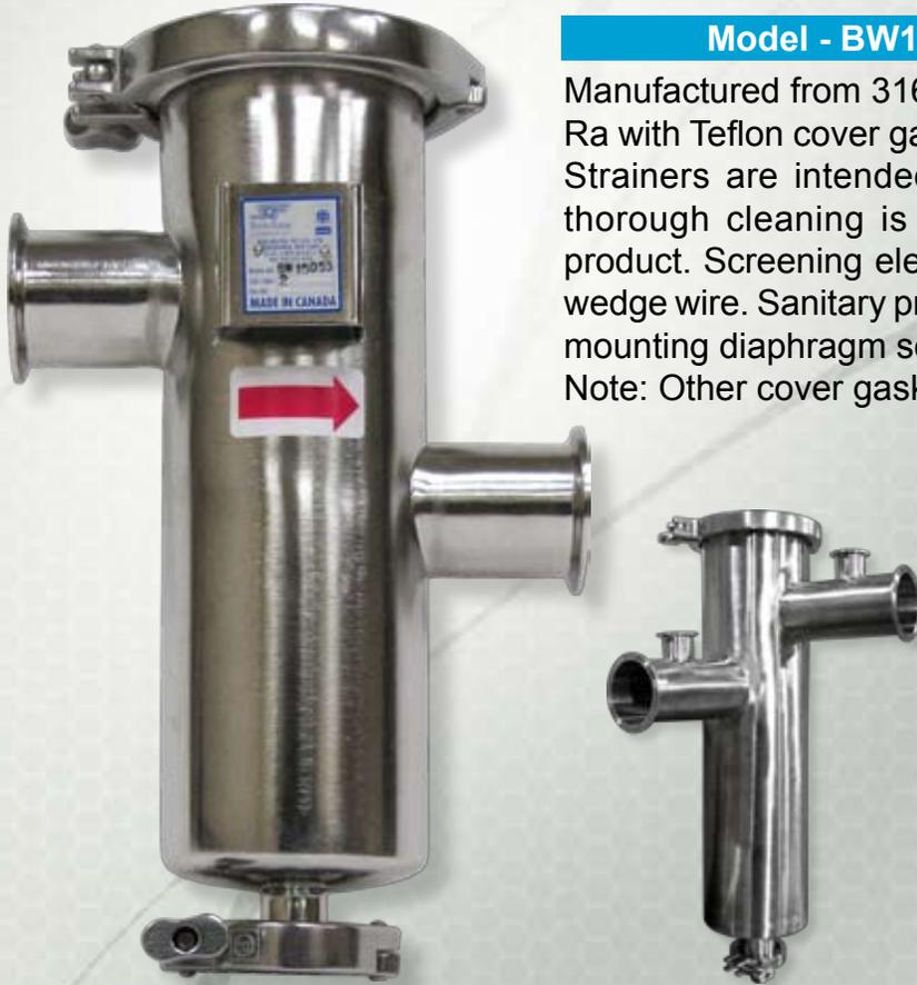
Manufactured from 316 Stainless Steel and polished to 25 Ra with Teflon cover gaskets. Sure Flow Try Clamp Basket Strainers are intended for applications where frequent, thorough cleaning is required between every batch of product. Screening elements include perforation, mesh or wedge wire. Sanitary pressure gauge ports are available for mounting diaphragm seals.
