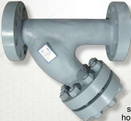
Sure Flow Class 1500 ASME Flanged Cast Y Strainers are available in both Carbon Steel and Stainless Steel. They provide economical protection for Water, Oil or Gas service. A machined, tapered seat ensures a perfect fit for the removable, stainless steel screen.
