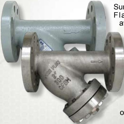
Sure Flow Class 300 ASME Flanged strainers are available in Carbon Steel and Stainless Steel. A machined, tapered seat ensures a perfect fit for the removable, stainless steel screen. All sizes come complete with flanged blow-off cover, gasket & plug. May be installed in vertical or horizontal pipelines with blow-off connection at the lower end of the screen.
