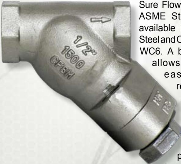
Sure Flow Class 1500 ASME Strainers are available in Stainless Steel and Chrome-Moly WC6. A bolted cover allows for quick, easy screen removal and a machined, tapered seat ensures a
