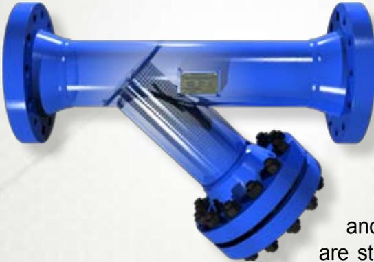
Sure Flow Fabricated "Y" Strainers can be designed to your specific application in Carbon Steel or Stainless Steel, along with other materials such as exotic alloys. Pipe sizes 2" to 24" in Class 150 and Class 300 ASME flanges are standard with the capability to supply larger pipe sizes and/or
