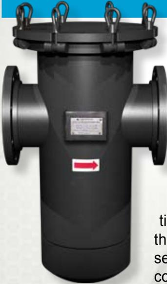
Sure Flow Fabricated Flanged Basket Strainers were initially developed for the petrochemical market. With continuous success they have now become a standard product available off the shelf in most sizes. The unique quick-opening closure and venting allows the field operator, in a timely and safe fashion, to remove the basket for cleaning. An o-ring seal provides positive sealing of the cover.
