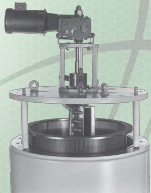
Figure 2 - The innovative internals of the Spyder-Clean showing ease of maintenance.
