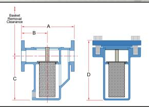
in the form of a basket, with a lifting handle, so that all particulate captured and retained by the screen can be easily removed for disposal. They are intended for applications where larger amounts of solid particulate are expected, and where clean-out will be frequent. Models are standard with a bolted "Swivel Clamp Cover" to allow fast and easy screen removal.
