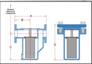
in the form of a basket, with a lifting handle, so that all particulate captured and retained by the screen can be easily removed for disposal. They are intended for applications where larger amounts of solid particulate are expected, and where clean-out will be frequent. Models are
