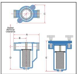
clean-out will be frequent. Models are standard with "Swivel Clamp Cover" to allow fast and easy screen removal without the use of tools. Covers have BUNA-N O-ring seals eliminating the need to change gaskets each time the strainer is serviced.
