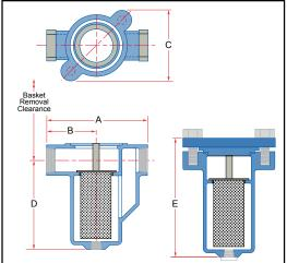
are expected, and where clean-out will be frequent. Models are standard with a bolted "Swivel Clamp Cover" to allow fast and easy screen removal with minimal tools. Covers have Viton O-ring seals, eliminating the need to change gaskets each time the strainer is serviced.
