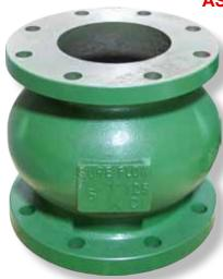
Sure Flow Globe Check Valves are designed to close before the pump stops completely. This prevents flow reversal which eliminates water hammer and system surges associated with valve closure. They feature quiet operation, a guided disc and can be installed in the vertical or horizontal position. The CF125ISC is offered in sizes ranging from 2" to 24".
