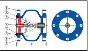
They feature quiet operation, a guided disc and can be installed in the vertical or horizontal position. The CF150C and CF150SSC are offered in sizes ranging from 2" to 12".
