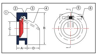
assures instantaneous closure to reversing flow, preventing build-up of momentum, which is the cause of damaging water hammer. The hinge pin design assures free movement of the disc and eliminates seizure under extreme conditions. A Buna-N soft seat insert on the CSW125IS is standard for positive sealing of hard-to-hold solvents and
