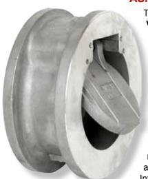
The Wafer Swing Check Valve incorporates several features distinguishing it from conventional check valves for silent, fast, non-slam operation. The most prominent of these is the accurately machined disc and its special quick closing action. Spring loading of the 316 Stainless Steel
