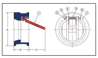
disc assures instantaneous closure to reversing flow, preventing build-up of momentum, which is the cause of damaging water hammer. The hinge pin design assures free movement of the disc and eliminates seizure under extreme conditions. Integral metal seat is standard for sealing. A lifting eye hook is standard on 8" to 14"
