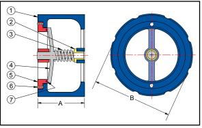
They feature quiet operation, a guided disc and can be installed in the vertical or horizontal position. The CW125ISC Wafer Check Valves are offered in sizes ranging from 2" to 12".
