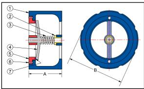
They feature quiet operation, a guided disc and can be installed in the vertical or horizontal position. The CW150C and CW150SS Wafer Check Valves are offered in sizes ranging from 2" to 12".
