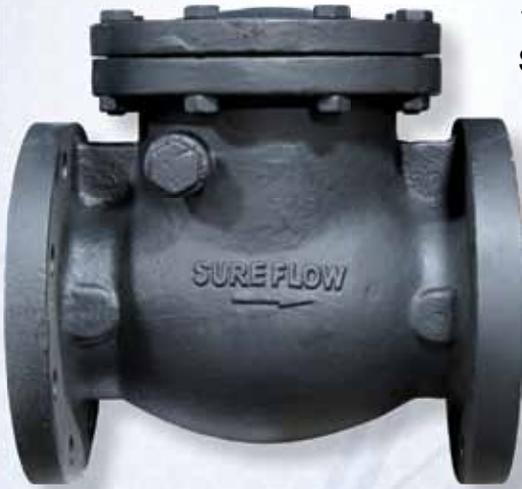
The Sure Flow **Horizontal Swing Check Valve** has a cast iron body, cover and disc. The valve is provided with a bronze seat ring and bronze disc ring. Bronze, being softer than a cast iron facing, offers a more positive sealing effect than competitors' standard iron facing. Furthermore, a bronze seat ring and bronze disc ring are used to ensure greater
