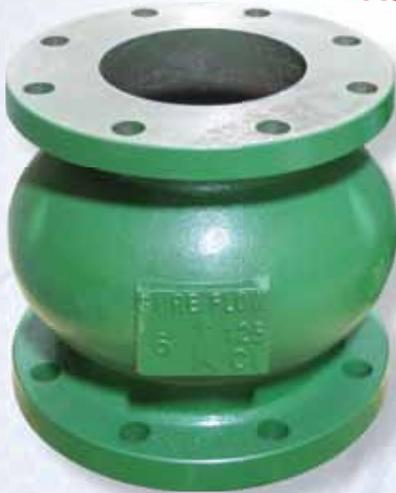
**Sure Flow Globe Check Valves** are designed to close before the pump stops completely. This prevents flow reversal which eliminates water hammer and system surges associated with valve closure. They feature quiet operation, a guided disc and can be installed in the vertical or horizontal position. The CF125ISC is offered in sizes ranging from 2" to 24".
