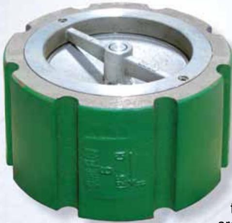
**Sure Flow Wafer Check Valves** are designed to close before the pump stops completely. This prevents flow reversal which eliminates water hammer and system surges associated with valve closure.
