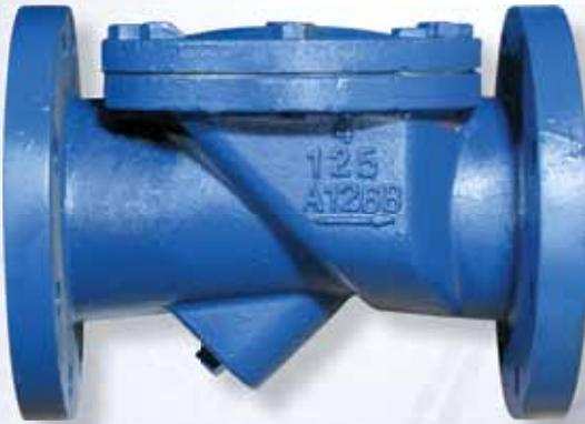
The **Elastic Swing Check Valve** is suitable for municipal and industrial applications. It is standard with a ductile iron body with ASME Class 125 flanges. The internal body is epoxy coated. The one-piece molded disc has a steel reinforced insert to ensure closure. Plus, while in the open position, it will allow 100% uninterrupted flow. The one-piece disc
