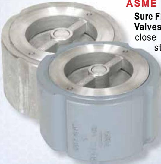
**Sure Flow Wafer Check Valves** are designed to close before the pump stops completely. This prevents flow reversal which eliminates water hammer and system surges associated with valve closure.
