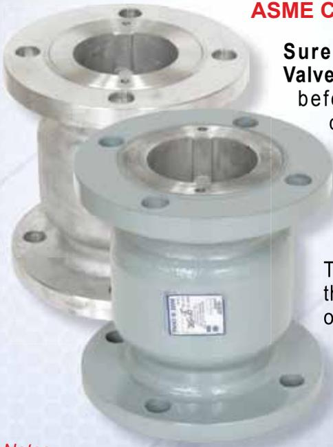
**Sure Flow Globe Check Valves** are designed to close before the pump stops completely. This prevents flow reversal which eliminates water hammer and system surges associated with valve closure.
