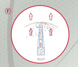
Port/straining element interface during backwashing cycle.
