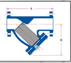
horizontal pipelines with blow-off connection at the lower end of the screen.
