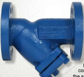
Sure Flow Ductile Iron Flanged Strainers feature a machined seat which ensures a perfect fit for the removable, stainless steel screen. All sizes come complete with flanged blow-off cover, gasket & plug. May be installed in vertical or horizontal pipelines with blow-off connection at the lower end of the screen.
