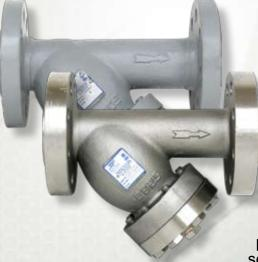
Sure Flow Class 600 ASME Flanged Cast Y Strainers are available in both Carbon Steel and Stainless Steel. They provide economical protection for Water, Oil or Gas service. A machined, tapered seat ensures a perfect fit for the removable. stainless steel screen.
