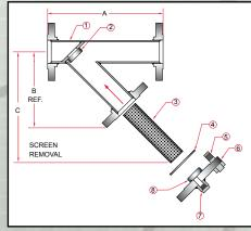
higher ASME pressure ratings. Screen sizes can be tailored to hold sufficient solids for the required time between clean-outs. Flange sizes can be chosen to fit existing piping, or to achieve the required clean pressure drop. Hinge covers are also available for quick opening. Please contact factory for details.
