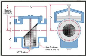
frequent clean-out of the basket is expected. Having a spare, clean basket on hand will greatly reduce the cleaning time, and differential pressure gauges, with alarms, can be supplied to get the maximum on-stream time between cleaning cycles.
