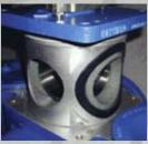
Should the diverter valve require service, it slides right out the top of the strainer body.
