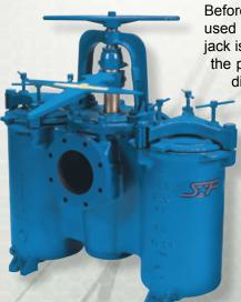
Before operating the handle a manual, integral lifting jack, built into the strainer is used to lift the diverter plug off of its seat. After the switching operation the lifting jack is used to reseat the plug. The lifting jack is specially designed to lift and seat the plug easily, even under high pressures. A built-in stop limits the distance the diverter plug can be raised. This minimizes the possibility of material bypassing
