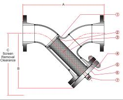
supply larger pipe sizes and/or higher ASME pressure ratings where needed. Screen sizes can be tailored to hold sufficient solids for the required time between clean-outs. Flange sizes can be chosen to fit existing piping, or to achieve the required clean pressure drop. Hinge covers are also available for quick opening. Alternate materials of construction are available. Please contact factory for details.
