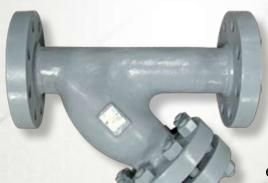
Sure Flow Class 900 ASME Flanged Cast Y Strainers are available inbothCarbon Steel and Stainless Steel. They provide economical protection for Water, Oil or Gas service. A machined, tapered seat ensures a perfect fit for the removable, stainless steel screen. These strainers may
