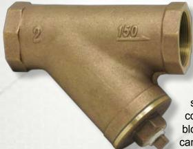
Sure Flow threaded strainers in Cast Bronze feature a machined, tapered seat which ensures a perfect fit for the removable, stainless steel screen. All sizes come complete with NPT blow-off with plug, which can be replaced with a ball
