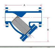
These strainers may be installed in vertical or horizontal pipelines with the blow-off connection at the lower end of the screen.
