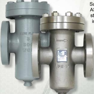
Sure Flow Class 300 ASME Flanged basket strainers are available in Cast Steel and Cast Stainless Steel. The screen is in the form of a basket, with a lifting handle, so that all particulate captured and retained by the screen can be easily removed for disposal.
