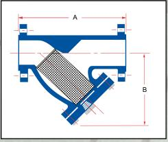
be installed in vertical or horizontal pipelines with the blow-off connection at the lower end of the screen.
