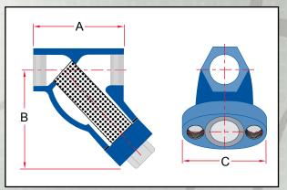
perfect fit for the removable stainless steel screen. This Strainer may be installed in vertical or horizontal pipelines with the blow-off connection at the lower end of the screen.
