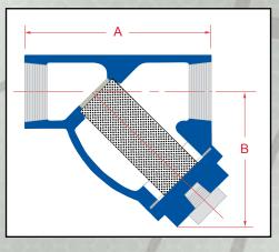
with blow-off and plug, which can be replaced with a ball valve for on-line blow-down of particulate.
