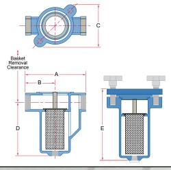
clean-out will be frequent. Models are standard with "Swivel Clamp Cover" to allow fast and easy screen removal without the use of tools. Covers have BUNA-N O-ring seals eliminating the need to change gaskets each time the strainer is serviced.
