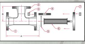
be fabricated with a standard bolted cover or a quick opening hinged cover (TWHA). The Sure Flow TWA Strainer can be fabricated to meet your specifications. The standard Strainer is constructed of Carbon or Stainless Steel material. Sure Flow also has vast experience in fabricating these strainers from Chrome-Moly material. Other materials, end connections and accessories are available.
