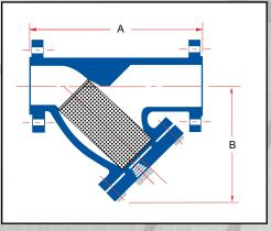
steel screen. These strainers may be installed in vertical or horizontal pipelines with the blow-off connection at the lower end of the screen.
