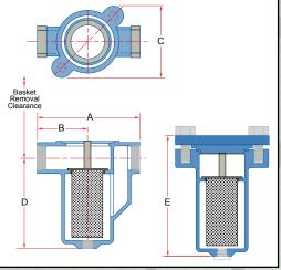
are expected, and where clean-out will be frequent. Models are standard with a bolted "Swivel Clamp Cover" to allow fast and easy screen removal with minimal tools. Covers have Viton O-ring seals, eliminating the need to change gaskets each time the strainer is serviced.
