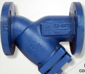
Sure Flow Cast Iron Flanged Strainers feature a machined seat which ensures a perfect fit for the removable, stainless steel screen. All sizes come complete with flanged blow-off cover, gasket & plug. May be installed in vertical or horizontal pipelines with blow-off connection at the lower end of the screen.
