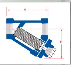
valve for on-line blow-down of particulate.
