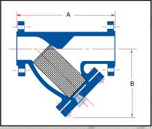
complete with solid threaded cover and gasket. May be installed in vertical or horizontal pipelines with blow-off connection at the lower end of the screen.
