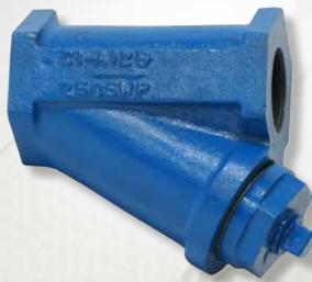
Sure Flow threaded strainers in Cast Iron feature a machined seat which ensures a perfect fit for the removable, stainless steel screen. All sizes come complete with NPT blow-off with plug, which can be replaced with a ball valve for on-line blow-down of particulate.
