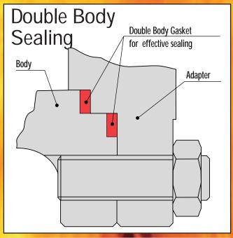
Double body gasket ensures positive body-joint sealing against pipeline stresses.
