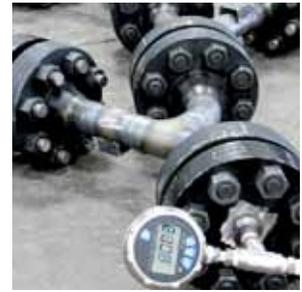
*To provide you with the most elite Strainer, Check valve, Butterfly valve, and a variety of other industrial valves, Sure Flow uses an in-house handheld PMI (Positive Material Identification) Analyzer. Within 5 seconds we can provide a full traceability of any alloy; plus download the analysis to provide an in-house M.T.R. (Material Test Report). We can even provide M.T.R. 's for welding rod, wire, pipe plugs and other raw materials.*
