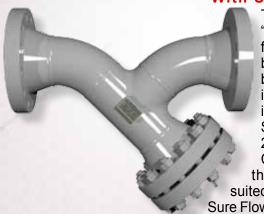
The Sure Flow Fabricated "FWT" Y strainer differs from the "FW" Y strainer by incorporating standard buttweld components into its construction. Fabricated in Carbon or Stainless Steel, pipe sizes 2" through 24" and in Class 150 and Class 300 ASME flanges,
