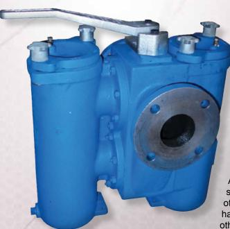
The duplex strainer has two separate strainer basket chambers. These chambers are put into service independently. When operating basket chamber shows a high pressure drop the flow is switched to the other one. The clogged basket chamber is then cleaned or replaced, ready for use again. Thus the duplex strainer can provide uninterrupted operation.
