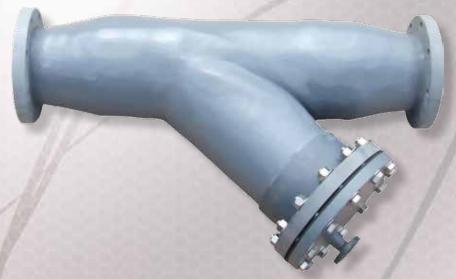
The lamination construction of FRP Strainers combines the chemical resistance of the particular liner material (thermoplastic) and the structural strength of fiberglass. Sure Flow Y Strainers are also offered in all-FRP construction. Resins can be used for high temperature and abrasive applications
