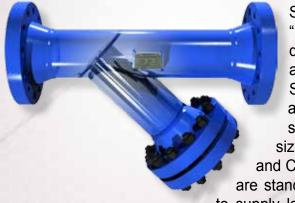
Sure Flow Fabricated "Y" Strainers can be designed to your specific application in Carbon Steel or Stainless Steel, along with other materials such as exotic alloys. Pipe sizes 2" to 24" in Class 150 and Class 300 ASME flanges
