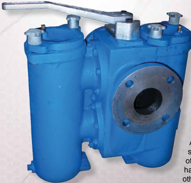
The duplex strainer has two separate strainer basket chambers. These chambers are put into service independently. When operating basket chamber shows a high pressure drop the flow is switched to the other one. The clogged basket chamber is then cleaned or replaced, ready for use again. Thus the duplex strainer can provide uninterrupted operation.
