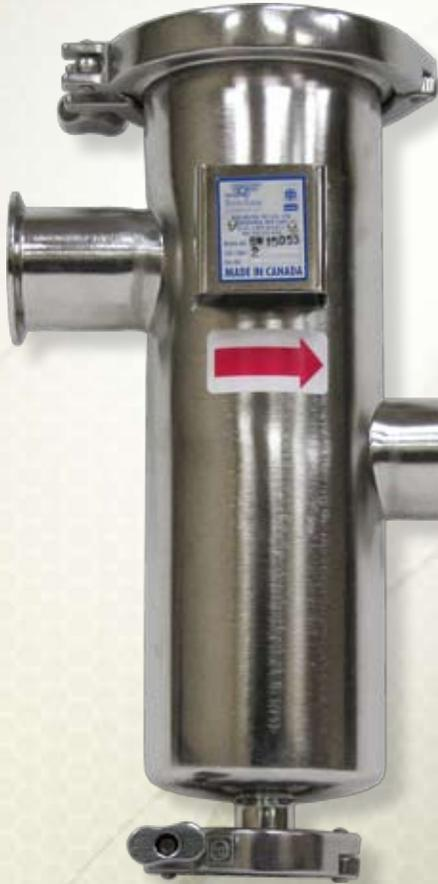
Manufactured from 316 Stainless Steel and polished to 25 Ra with Teflon cover gaskets. Sure Flow Try Clamp Basket Strainers are intended for applications where frequent, thorough cleaning is required between every batch of product. Screening elements include perforation, mesh or wedge wire. Sanitary pressure gauge ports are available for mounting diaphragm seals.
